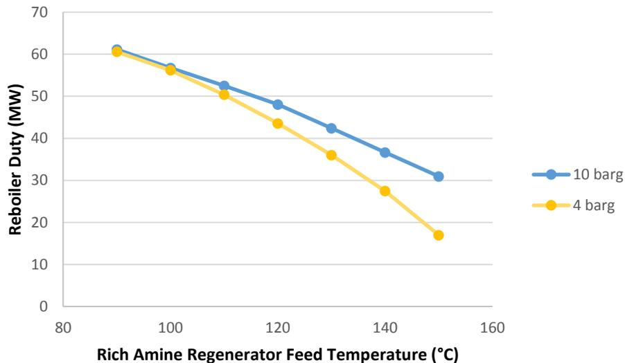
**Figure 13: The Effect of the Rich Amine Temperature and the Flash Temperature on the Reboiler Duty for DGA<sup>®</sup>**
