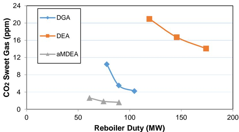
**Figure 3: CO<sub>2</sub> Content in Sweet Gas with Varying Reboiler Duty Using Different Amines at Maximum Absorber Loading**
