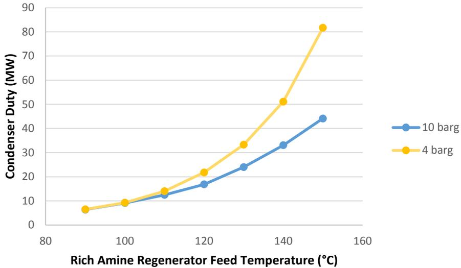
**Figure 14: The Effect of the Rich Amine Temperature and the Flash Temperature on the Condenser Duty for DGA®**
