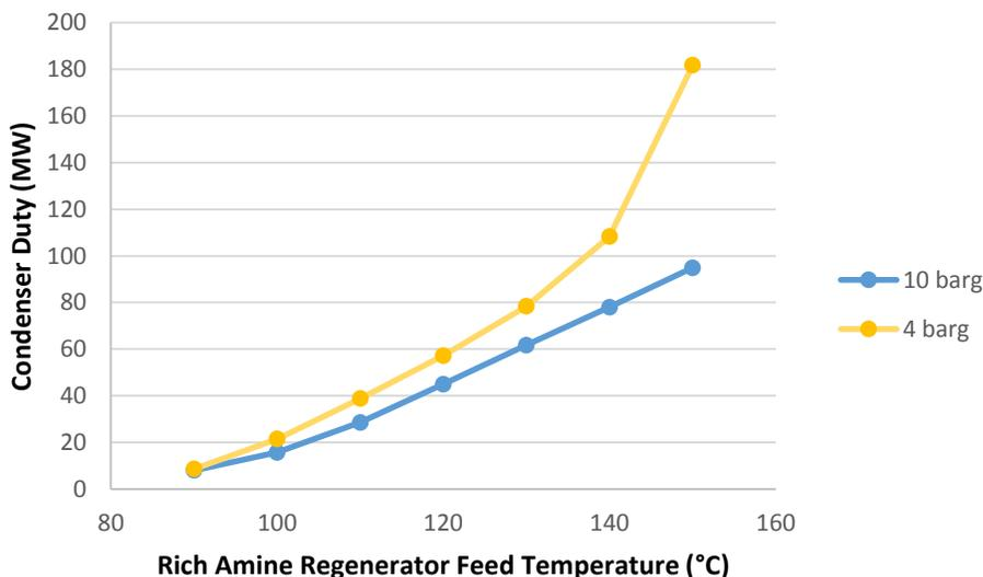
**Figure 16: The Effect of the Rich Amine Temperature and the Flash Temperature on the Condenser Duty for MDEA**
