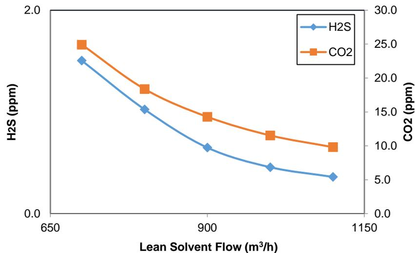
Figure 8: DGA<sup>®</sup> Circulation Rate Effect on H<sub>2</sub>S and CO<sub>2</sub> in the Sweet Gas
