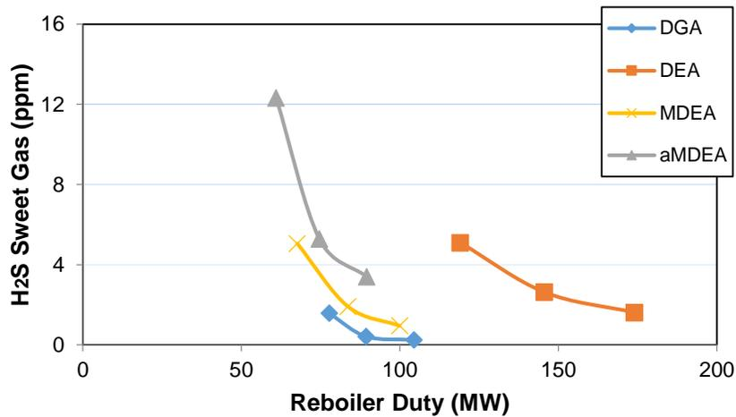
**Figure 2: H<sub>2</sub>S Content in Sweet Gas with Varying Reboiler Duty Using Different Amines at Maximum Absorber Loading**
