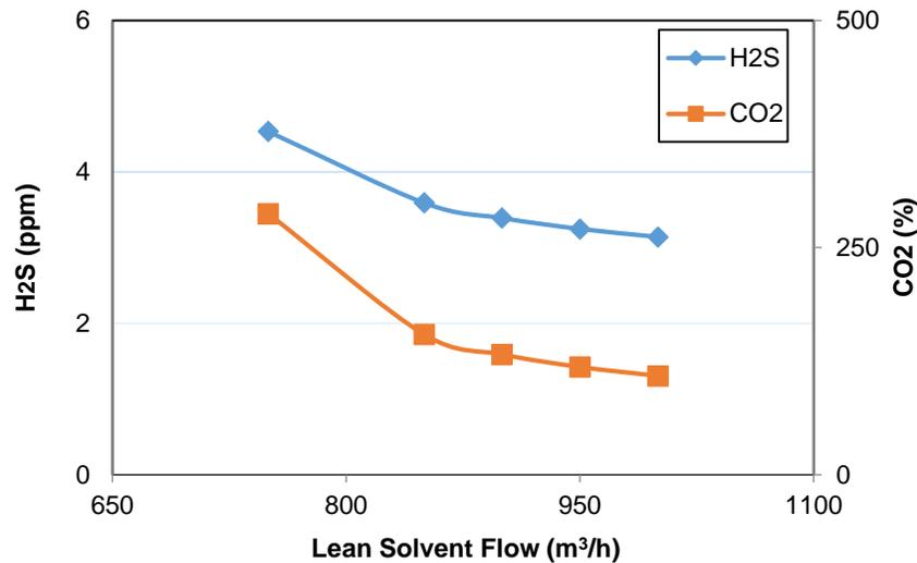
**Figure 9: MDEA Circulation Rate Effect on H<sub>2</sub>S and CO<sub>2</sub> in the Sweet Gas with 1.1 lb/gal Steam Ratio**
