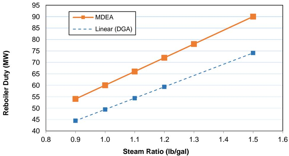
Figure 12: The Relationship between Steam Ratio and Reboiler Duty for MDEA (850 m<sup>3</sup>/hr) and DGA<sup>®</sup> (700 m<sup>3</sup>/hr)
