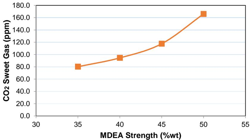
Figure 6: MDEA Concentration Effect on CO<sub>2</sub> Absorption
