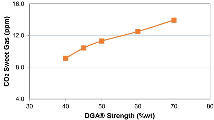
Figure 5: DGA® Concentration Effect on CO<sub>2</sub> Absorption
