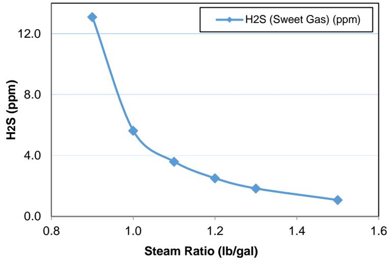
**Figure 10: Effects of Steam Ratio (lb of steam for reboiler: gallons of amine circulated) on H<sub>2</sub>S Content in Sweet Gas**
