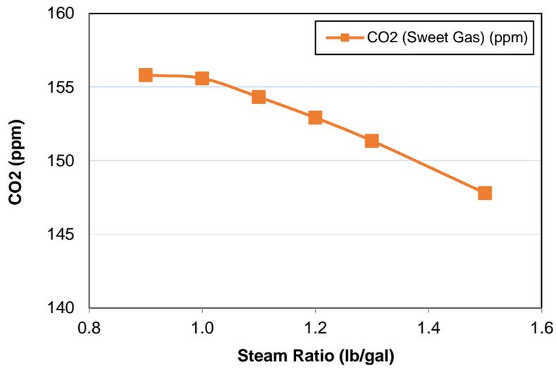
Figure 11: Effects of Steam Ratio (lb of steam for reboiler: gallons of amine circulated) on CO<sub>2</sub> Content in Sweet Gas
