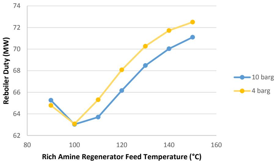
**Figure 15: The Effect of the Rich Amine Temperature and the Flash Temperature on the Reboiler Duty for MDEA**
