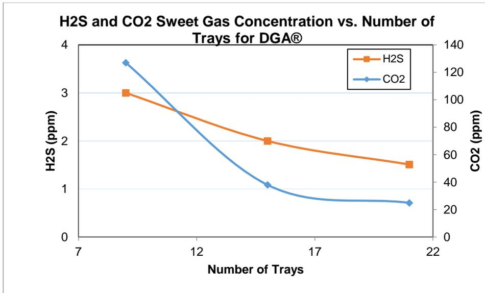
Figure 17: The Effect of the Number of Trays on the Acid Gas Absorption in the Absorber for DGA®
