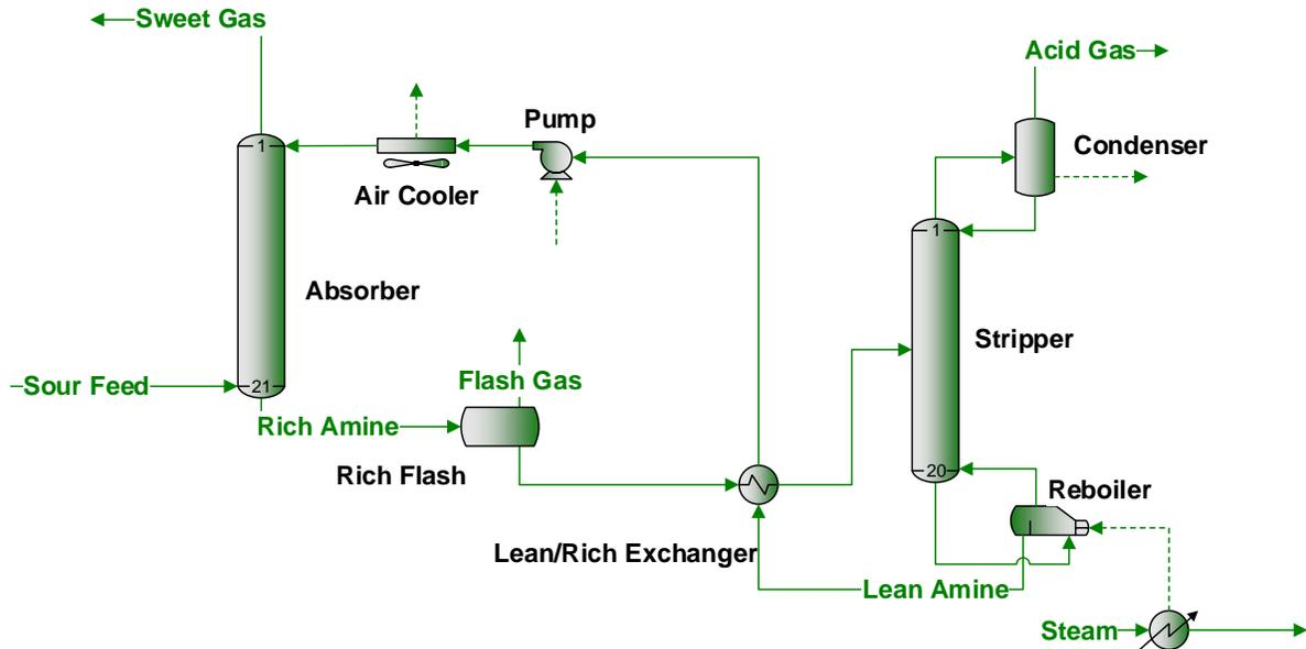
Figure 1: Flow Diagram for Typical Amine Sweetening Unit
