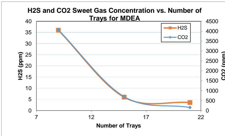
Figure 18: The Effect of the Number of Trays on the Acid Gas Absorption in the Absorber for MDEA
